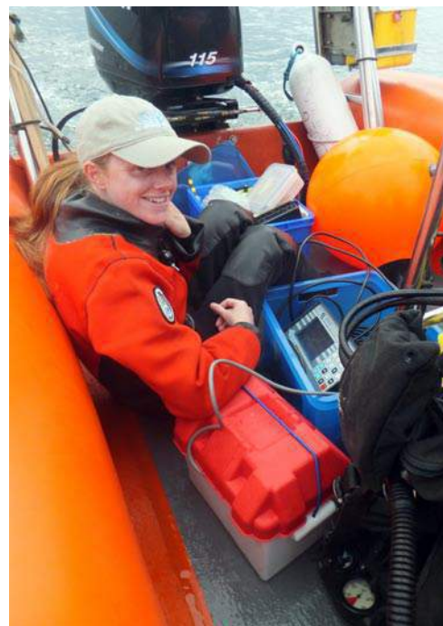
Figure 4: Aquascan AX2000 proton magnetometer deployed from a small inflatable boat
